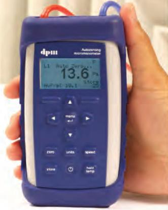
With a multi-function white LED back lit display, the auto ranging, auto-zeroing manometer is able to give true pressure, velocity and live volume readings with optional temperature measurement using K type probes, with high accuracy.
